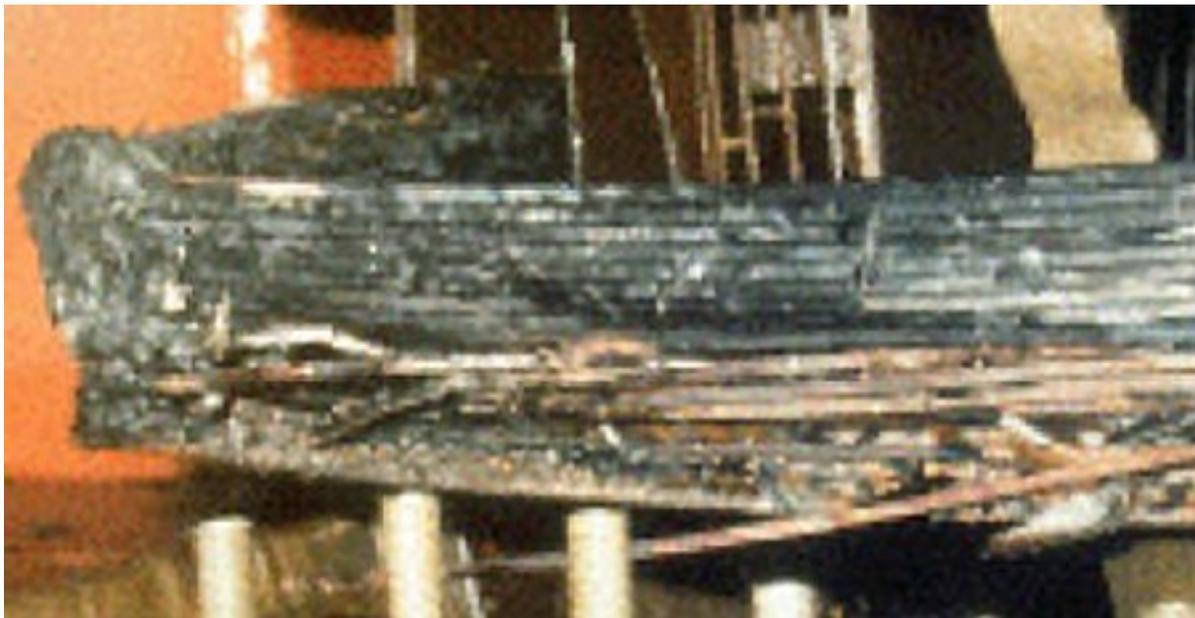
**Melted low voltage winding at 345 kV GSU transformer, Seabrook Station, NH, during mild solar storm with reversal of electrojets, transformer saturation, vibration of stainless steel bolt, damage to Phase A transformer, Nov. 10, 1998, 12.2 day outage.**
