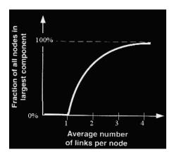
Paul Erdos' "small world" network theory applies to EMP failure analysis.<sup>11</sup> The graph above illustrates that the average fraction of nodes in any network that are connected to any single network node changes suddenly when the average number of links per node exceeds one. For example, a failed node, where the average links per node is 2, can affect ~ 50% of the remaining network nodes.
