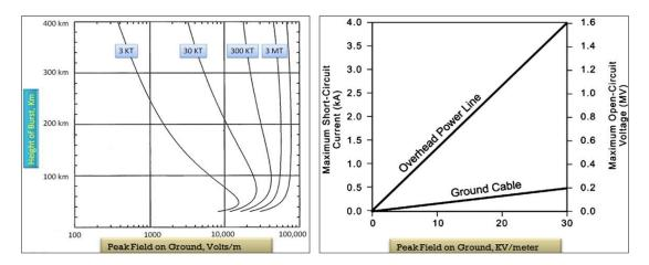
The first graph above illustrates that nominal weapons with yields ranging from 3 kilotons to 3 megatons (a 3 order of magnitude difference in yield), exhibit a range of peak E1 fields on the ground with only a factor of 3 difference, i.e. 15kV/meter vs. 50 kV/meter. Although E3 fields vs. yield and height of burst are not illustrated above, a 30 kiloton nuclear weapon detonated
