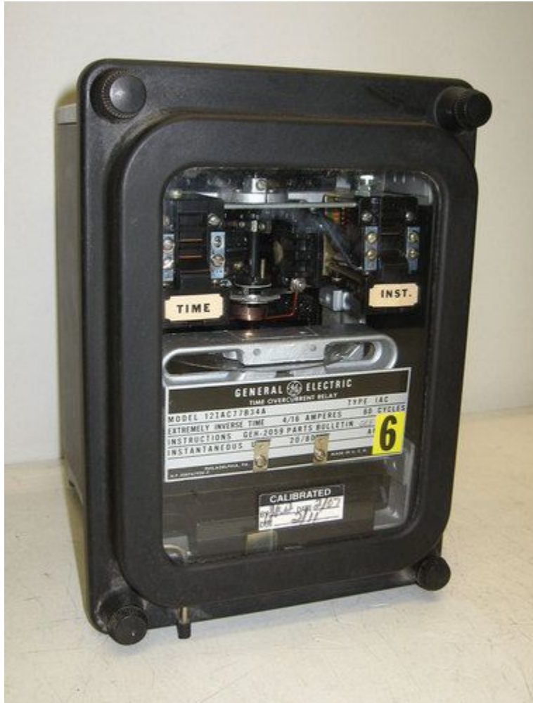
Figure 32: Vintage Electromechanical Relay. Electromechanical relays such as the General Electric model pictured here were once widely installed in substations, but now represent a minority of relays in use. Testing shows these devices are resilient to the E1 pulse. Photo credit: Pinterest/MCBIA Sales .
