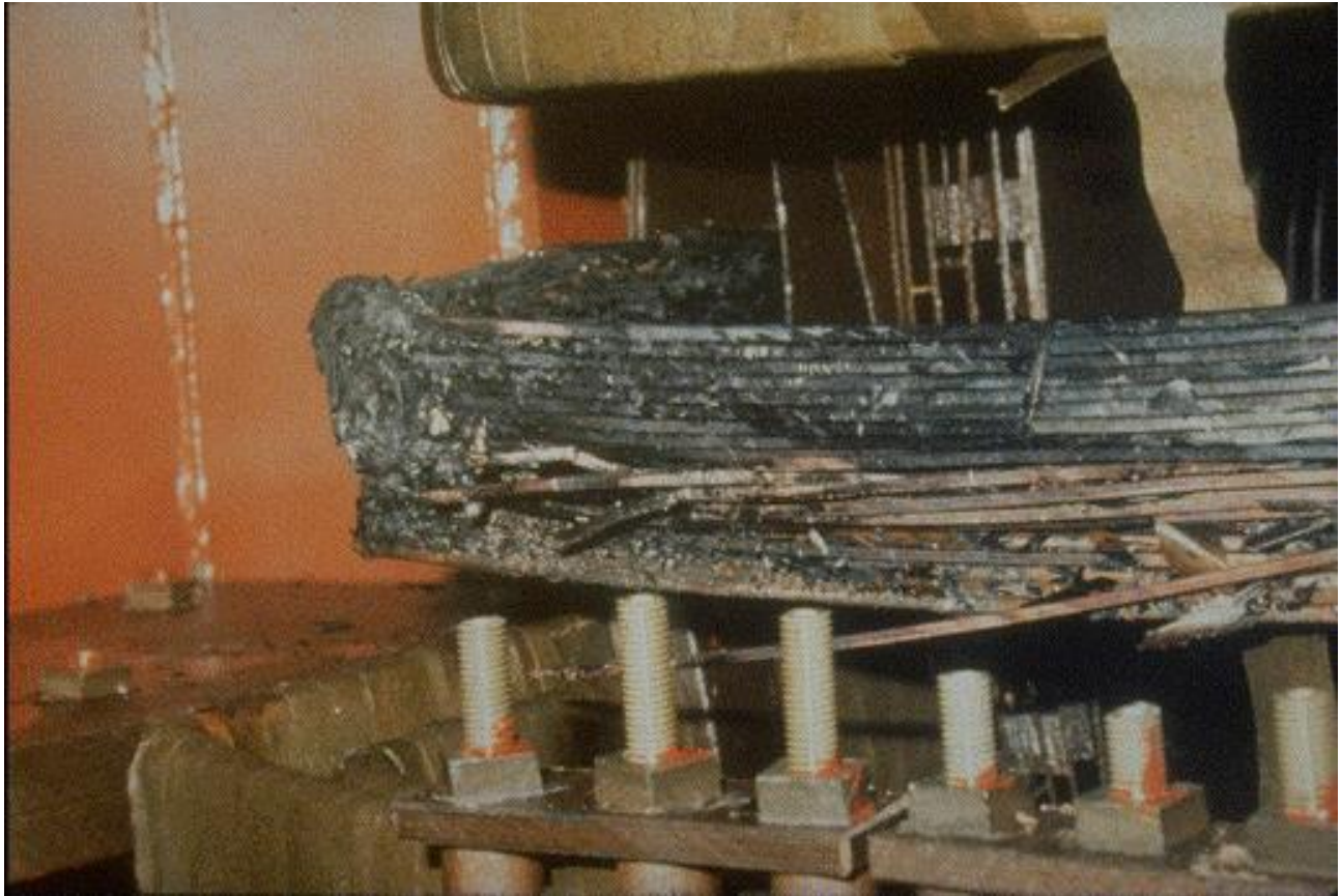
Figure 2: Melted Windings of Phase 1A Transformer at Salem Nuclear Plant in New Jersey in Aftermath of March 1989 Solar Storm
